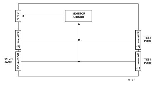
Figure 2-11. PSM-12 Test Module with LED Monitoring
